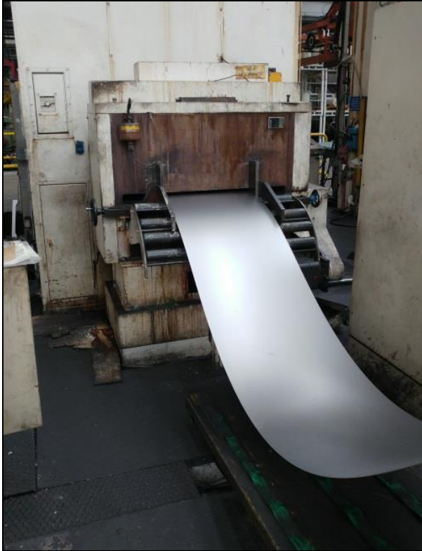
N. 1 SEMI-COMPACT FEEDING LINE FOR PRESSES YEAR 1988 N. 1 SEMI-COMPACT FEEDING LINE FOR PRESSES YEAR 1988
