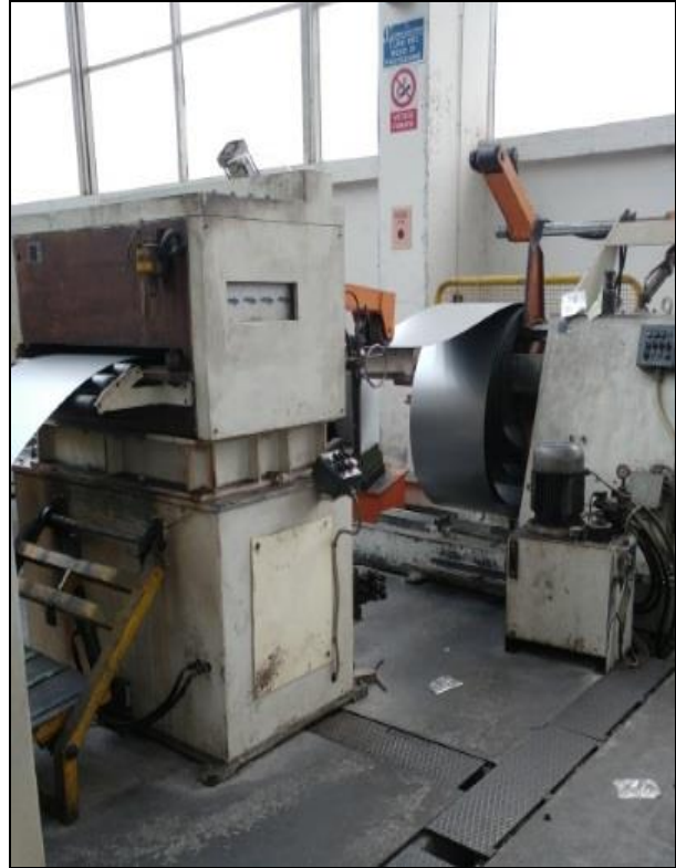
N. 1 SEMI-COMPACT FEEDING LINE FOR PRESSES YEAR 1988 N. 1 SEMI-COMPACT FEEDING LINE FOR PRESSES YEAR 1988
